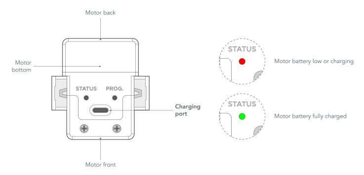
The motor has a USB-C charging port on the bottom. To charge the motor's battery, simply plug the charging cable into the charging port. A full charge typically takes around 8 hours if the battery is fully depleted. Whilst charging, the STATUS light on the bottom of the motor will glow red, then change to green when fully charged.
