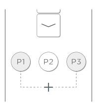
Press and hold the P1 and P3 buttons together until the motor 'jogs'. The motor is now in configuration mode.
