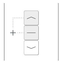
Hold the OPEN and STOP buttons until the motor 'jogs'. The motor is now deleted from that channel.
