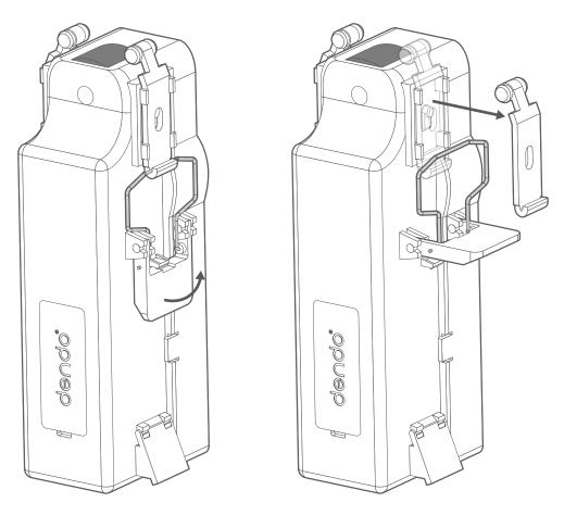
Start by unclipping one of the runners from the top of the motor. Lift the retaining clip then simply pull the runner free of its mounts on the side of the motor.
