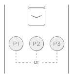
Press and hold either P1, P2 or P3 until the motor 'jogs'. The new intermediate stop-point is now set to that button.
