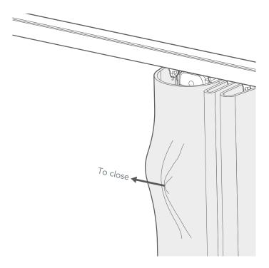
To open the curtains once the motor is installed, simply take the leading edge of the curtain and give it a sharp but gentle pull in the direction you want the curtain to open. The motor will detect the movement and engage, opening the curtain until fully open. To close the curtains, simply pull the leading edge of the curtain in the opposite direction.
