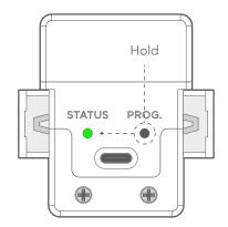
On the bottom of the motor, press and hold the PROG. button until the STATUS light turns green.
