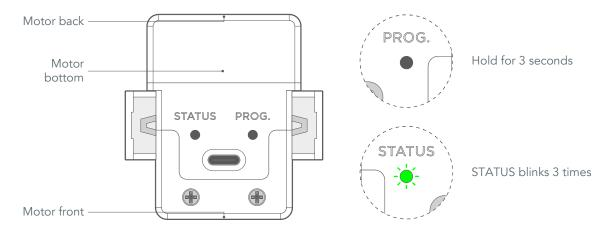
The motor is in its 'deep sleep' state when it is sent to you and will not operate until it is removed from this state. To do so, simply press and hold the PROG. button on the bottom of the motor for around 3 seconds, until the STATUS light blinks 3 times. The motor is now operational.
