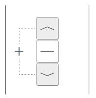
Hold the OPEN and CLOSE buttons on the remote at the same time until the motor 'jogs' briefly.
